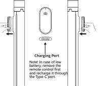
Install the remote contro Remove the remote control The remote control is absorbed by the magnet and taken out. When putting it back, align it at the slot and adsorb automatically.
