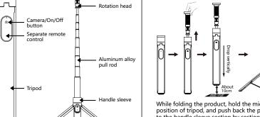
While folding the product, hold the middle position of tripod, and push back the pull rod back to the handle sleeve section by section.
