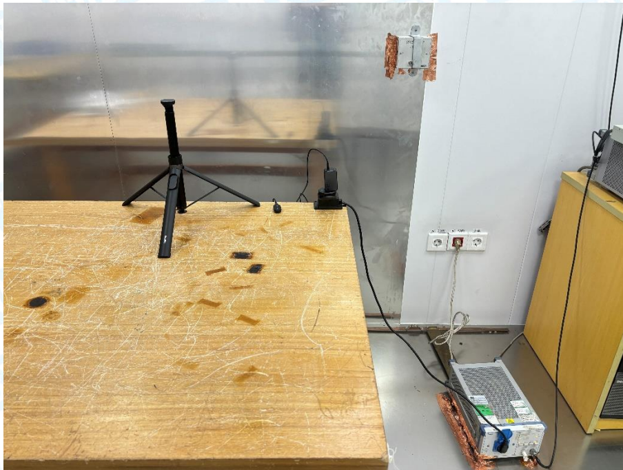
Photo of Setup for Conducted Emission
