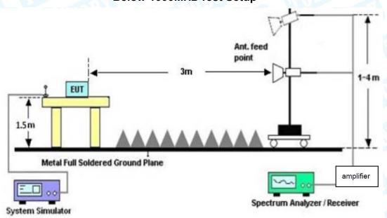
**Above 1GHz Test Setup**
