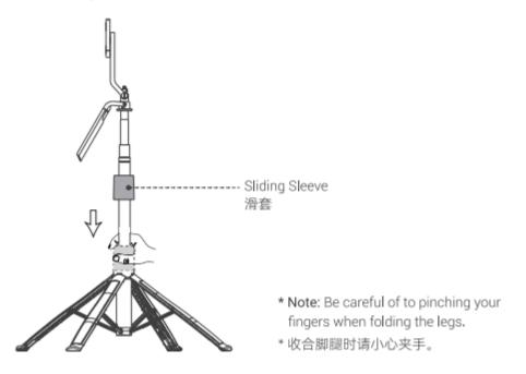
5. Extend the telescopic pole to the desired height. 拉开伸缩杆至所需高度。
