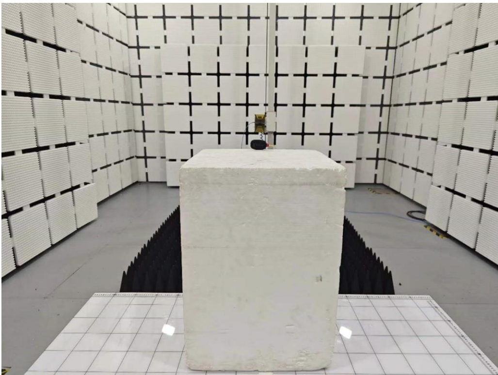
Set-up for Radiated Spurious Emission, Above 1GHz
