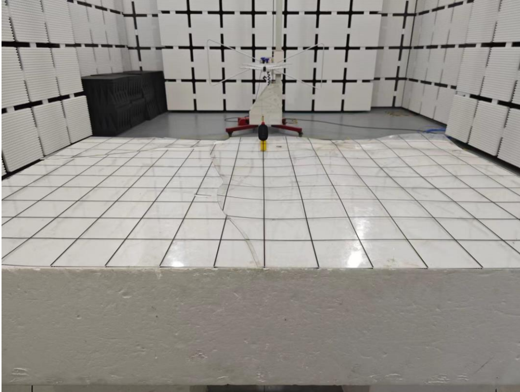
Set-up for Radiated Spurious Emission, Above 1GHz
