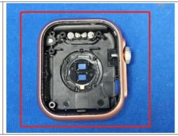
The antenna is LAP Bluetooth antenna.
