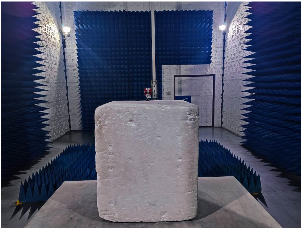
RADIATED EMISSION TEST SETUP ABOVE 1GHz
