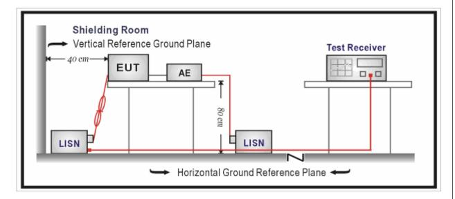
Note: AC Power source is used to change the voltage 120V/60Hz.
