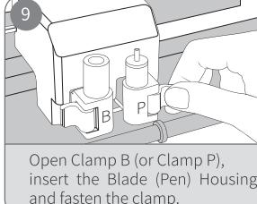
Open Clamp B (or Clamp P), insert the Blade (Pen) Housing and fasten the clamp.
