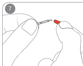
Take out the Blade Housing and a blade, and take off the blade's protective shell. (The red Fine-Point Blade is recommended.)
