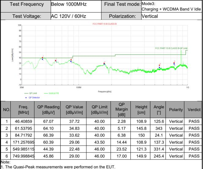
2. Value = Reading(dB<sub>µ</sub>V) + AF(dB/m) + Factor(dB):
