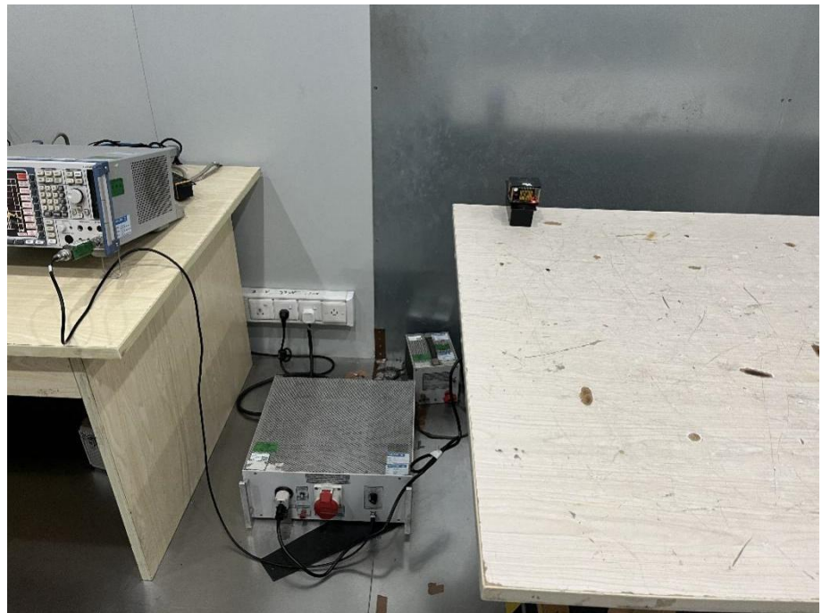
Conducted Emission Test Setup
