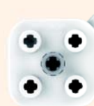
Connected to the 3-pin port and spins after started
