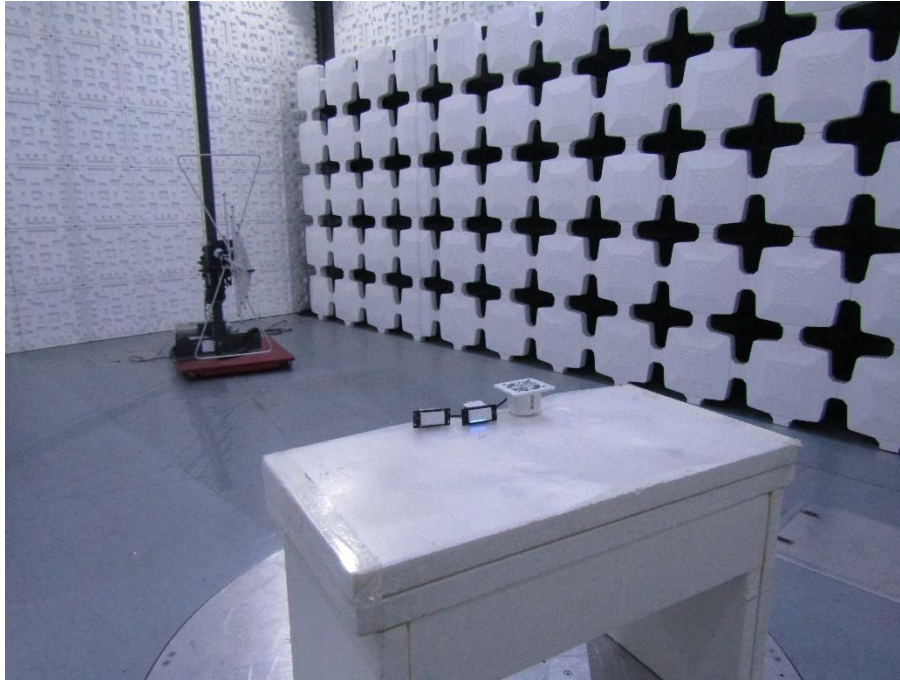
Radiated Emission (Above 1GHz)
