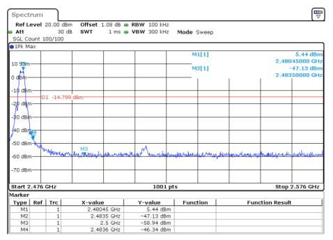
Note: This line in the plots is a reference line for the 20dB down limit, not the limit.
