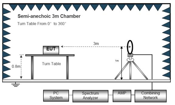
(B) Radiated Emission Test-Up Frequency 30MHz~1GHz
