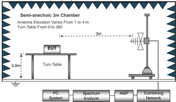
(C) Radiated Emission Test-Up Frequency Above 1GHz
