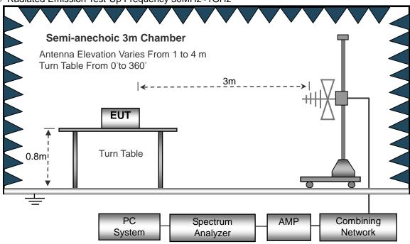
(C) Radiated Emission Test-Up Frequency Above 1GHz
