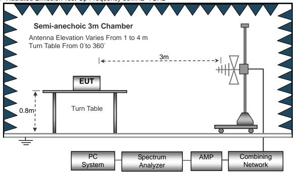
(C) Radiated Emission Test-Up Frequency Above 1GHz
