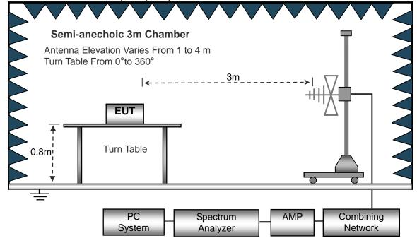
(C) Radiated Emission Test-Up Frequency Above 1GHz
