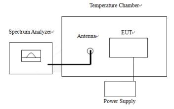
The EUT which is powered by the Battery, is coupled to the Spectrum Analyzer; the RF load attached to the EUT antenna terminal is 500hm; the path loss as the factor is calibrated to correct the reading 5.4 EUT OPERATION CONDITIONS
