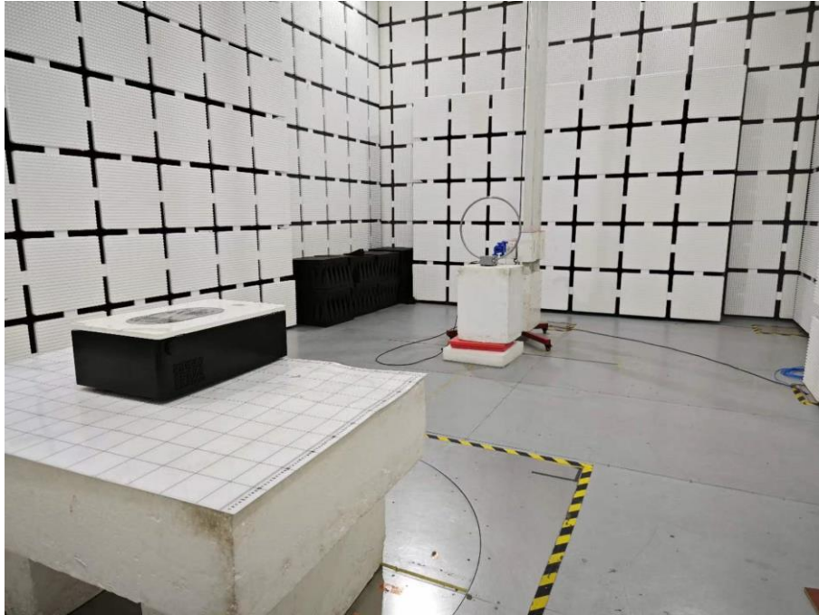
Set-up for Radiated Spurious Emission, Above 1GHz
