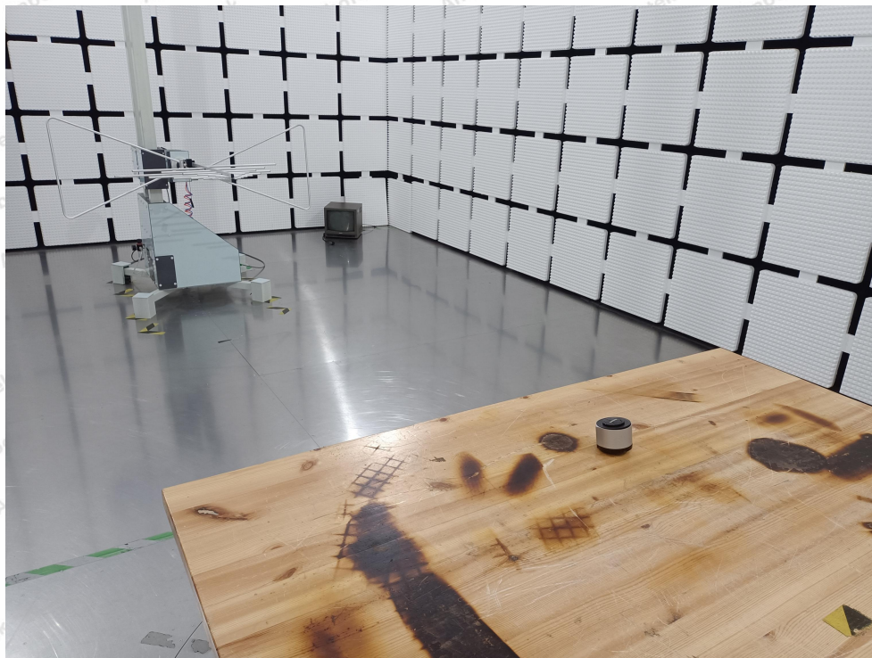
Photo of Radiation Emission Test
