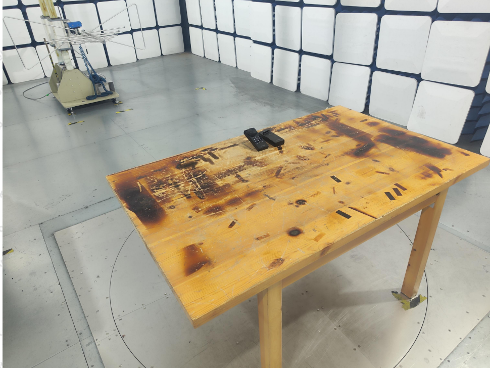
Photo of Radiation Emission Test (below 1GHz)
