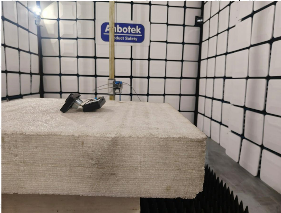
Photo of Radiation Emission Test (above 1GHz)
