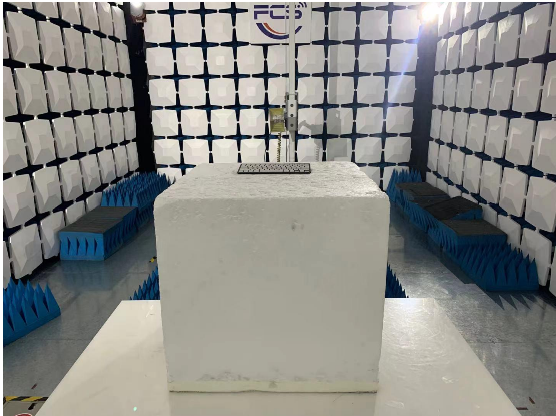
Above 1GHz for radiated emission test setup
