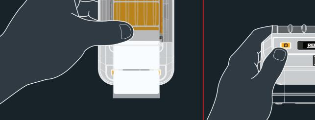
Press and release the Power ON/OFF button (left side button) until sound is heard and REEKON logo appears on the OLE display.
