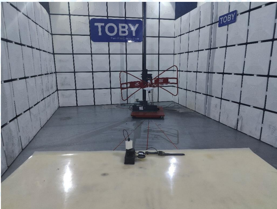
Photo of Setup for Radiated Emission (30MHz~1GHz)
