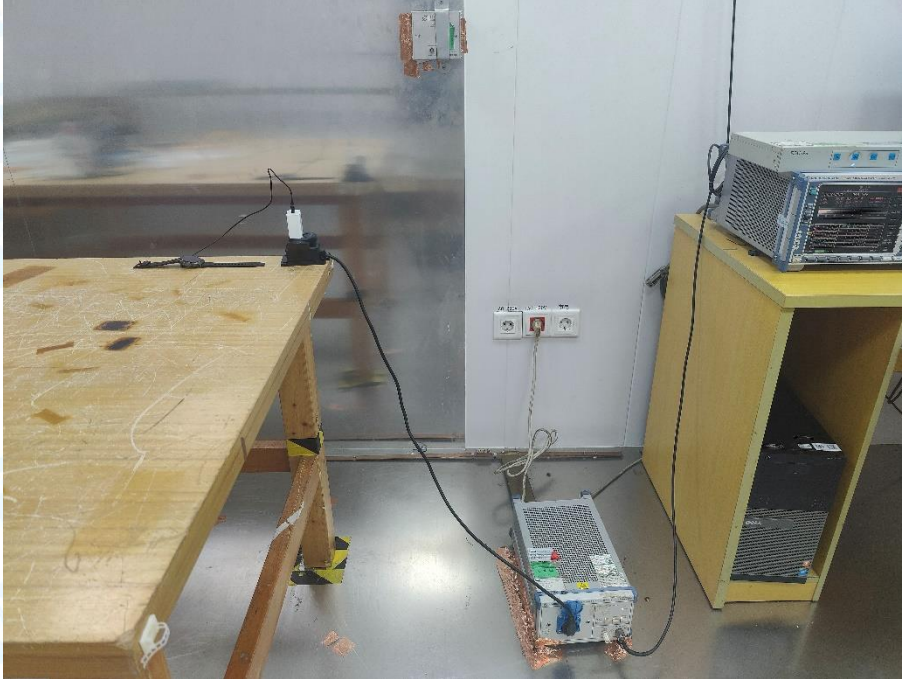
Photo of Setup for Radiated Emission (30MHz~1GHz)
