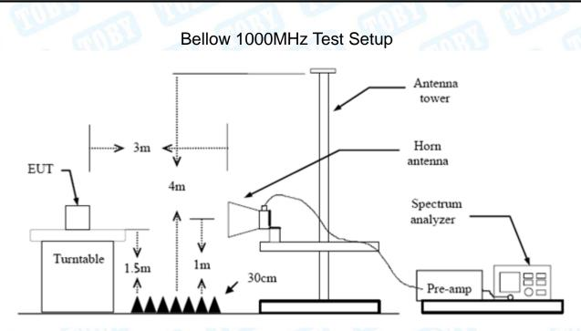
Above 1GHz Test Setup
