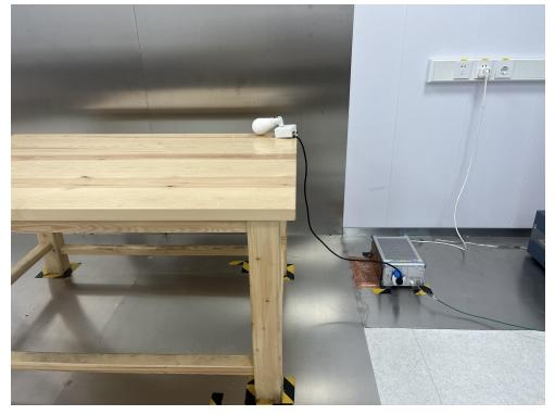
Radiated Emission Test View|(Below 1G)
