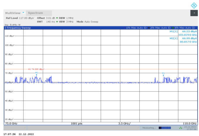
Figure 8.4-6: Radiated spurious emissions within 75–110 GHz
