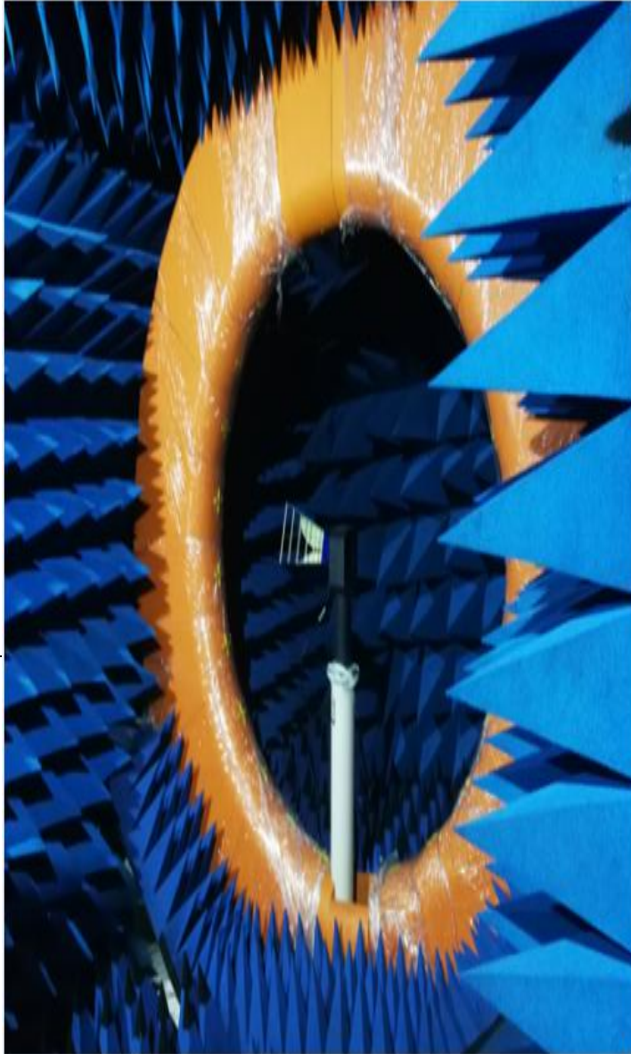
24-probe microwave chamber
