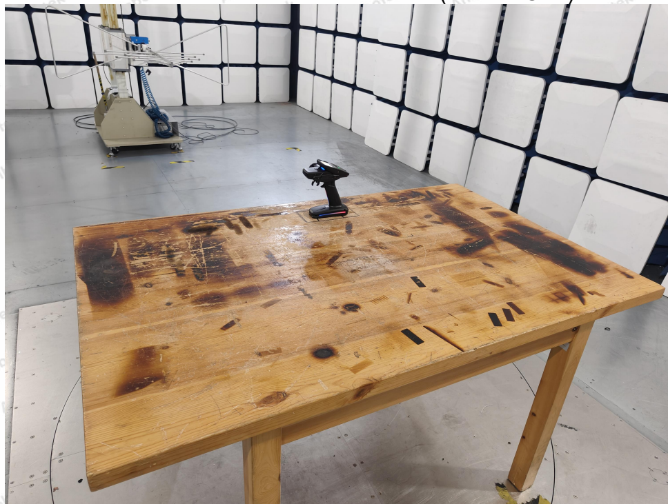
Photo of Radiation Emission Test (below 1GHz)
