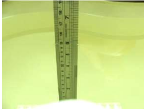
Photo of Liquid Height for Head SAR
