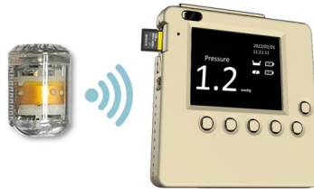
Step4. Recording Pressure & Temperature
