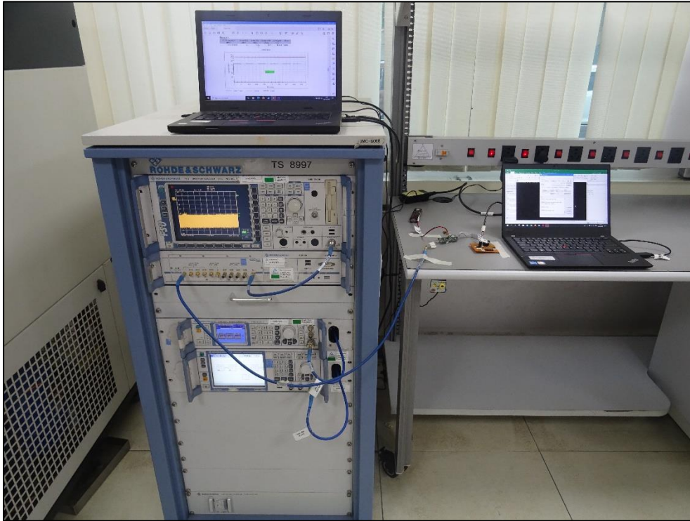
Antenna Port Measurement Test Setup
