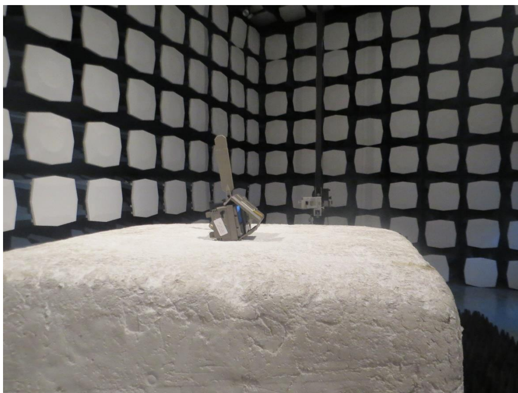
Picture 1: Radiated Spurious Emissions Test setup
