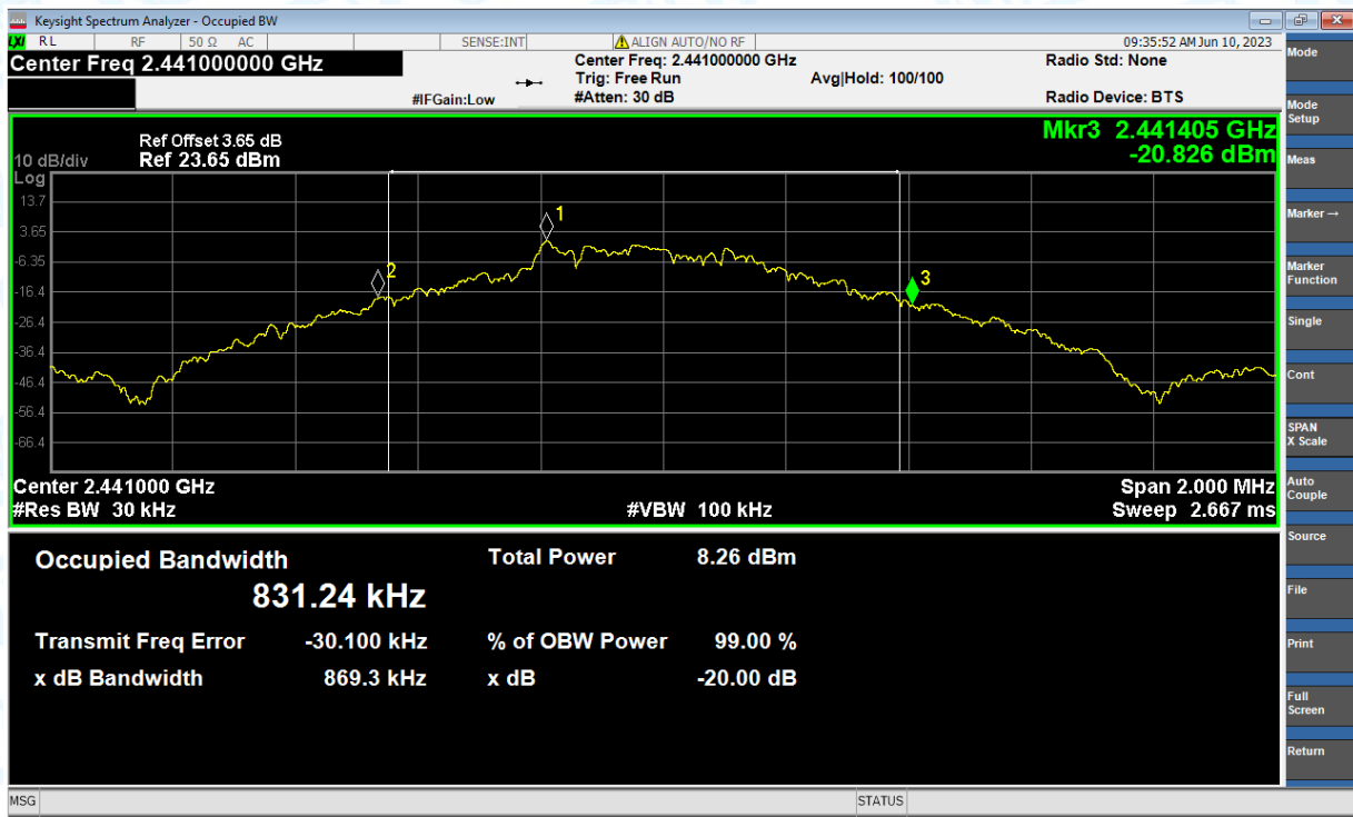
-20dB Bandwidth NVNT 1-DH1 2441MHz Ant1
