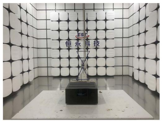
Radiated Test (Above 1GHz)
