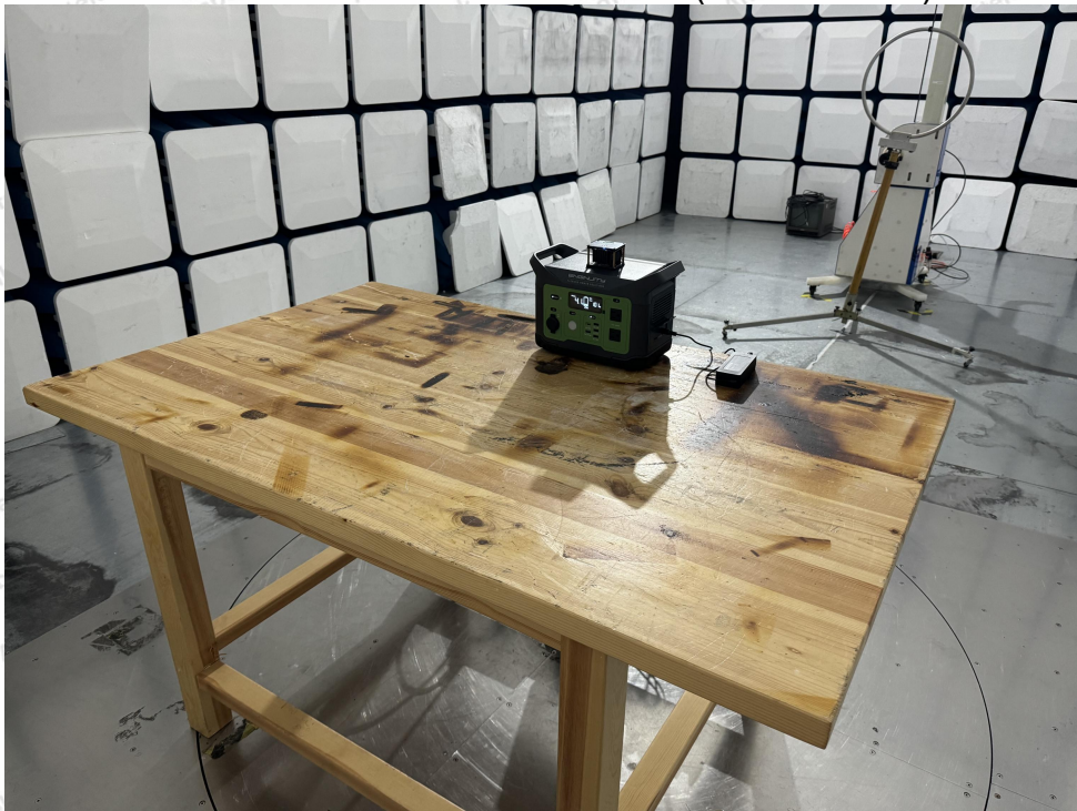
Photo of Radiation Emission Test (below 30MHz)
