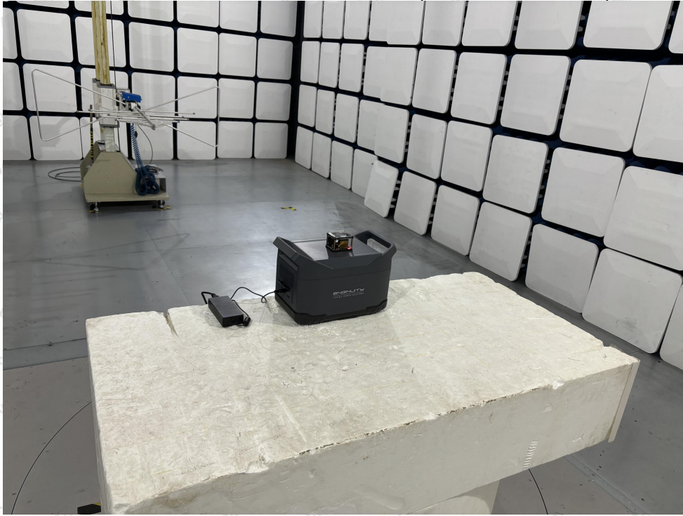
Photo of Radiation Emission Test (30MHz~1000MHz)
