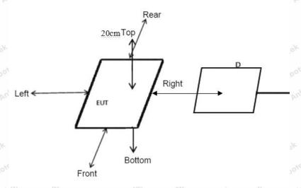
Note: Measurements should be made at 20 cm surrounding the EUT and 20cm above the top surface of the EUT.
