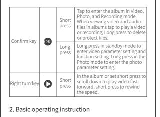
Long press the " O " key to power on the device when the device is powered off. The LCD is on and an announcement is heard. (2)Turn off the machine Long press the " O " button to turn off the machinein any mode
