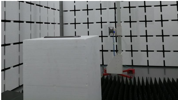
Radiated emission above 1GHz
