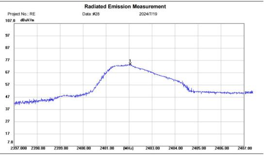
Site Polarization: Vertical Temperature: (C)
