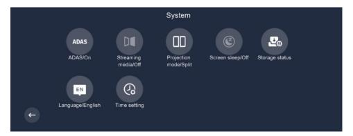
a. ADAS: When the switch is on, the system will make the appropriate warning judgement based on the vehicle ahead, the lane departured and the position of the vehicle and broadcast(the car started, the lane departured, attention to the front car); when the switch is off, no
