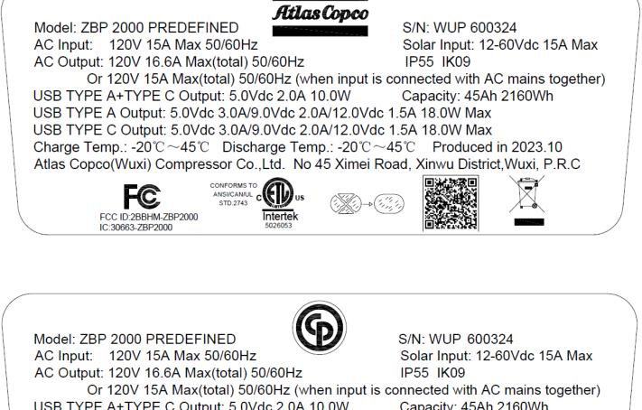
USB TYPE A+TYPE C Output: 5.0Vdc 2.0A 10.0W Capacity: 45Ah 2160Wh USB TYPE A Output: 5.0Vdc 3.0A/9.0Vdc 2.0A/12.0Vdc 1.5A 18.0W Max USB TYPE C Output: 5.0Vdc 3.0A/9.0Vdc 2.0A/12.0Vdc 1.5A 18.0W Max Charge Temp.:  $-20^{\circ}$ C  $\sim 45^{\circ}$ C Discharge Temp.:  $-20^{\circ}$ C  $\sim 45^{\circ}$ C Produced in 2023.10 Atlas Copco(Wuxi) Compressor Co.,Ltd. No 45 Ximei Road, Xinwu District,Wuxi, P.R.C
