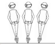
On not turn the handlebar sharply at high speeds.
