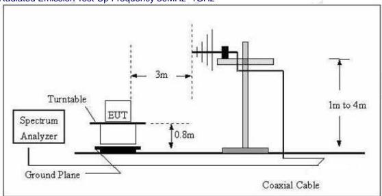
(C) Radiated Emission Test-Up Frequency Above 1GHz
