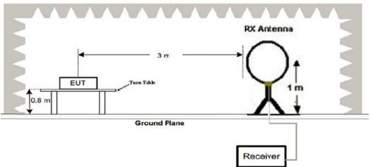
2. Radiated Emission Test-Up Frequency 30MHz~1GHz
