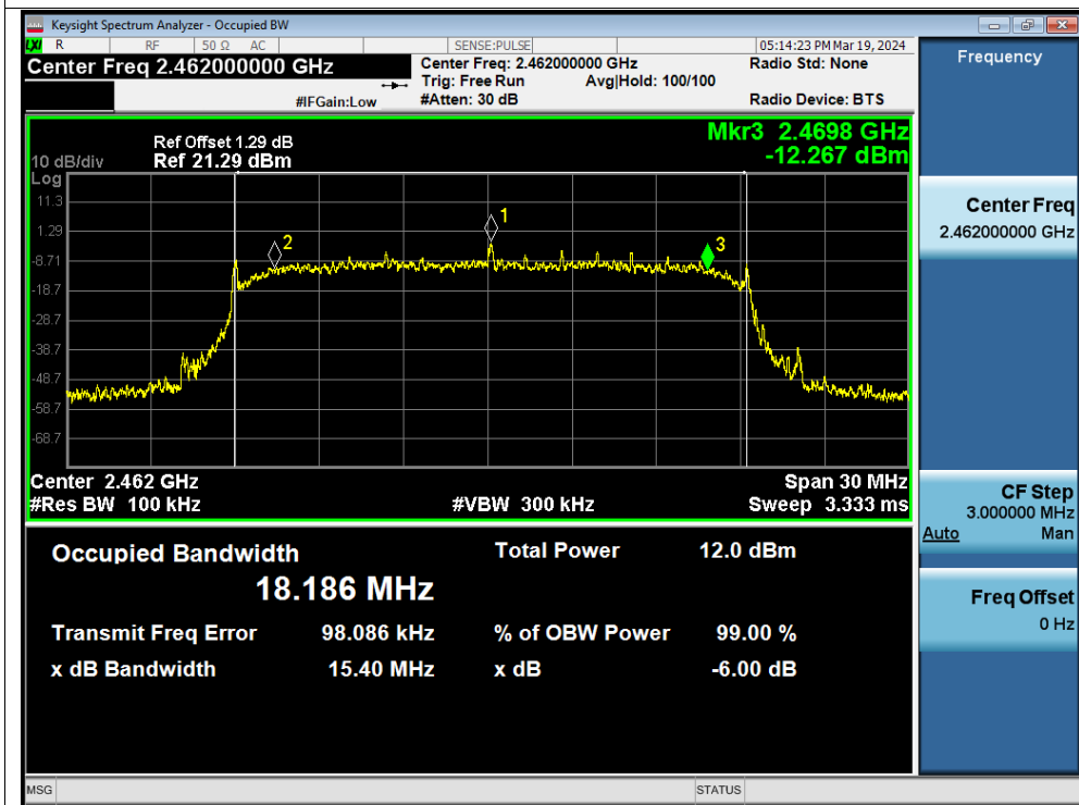
-6dB Bandwidth NVNT n40 2422MHz Ant1
