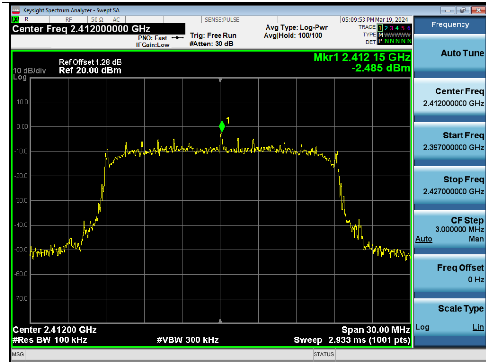
Tx. Spurious NVNT n20 2412MHz Ant1 Emission
