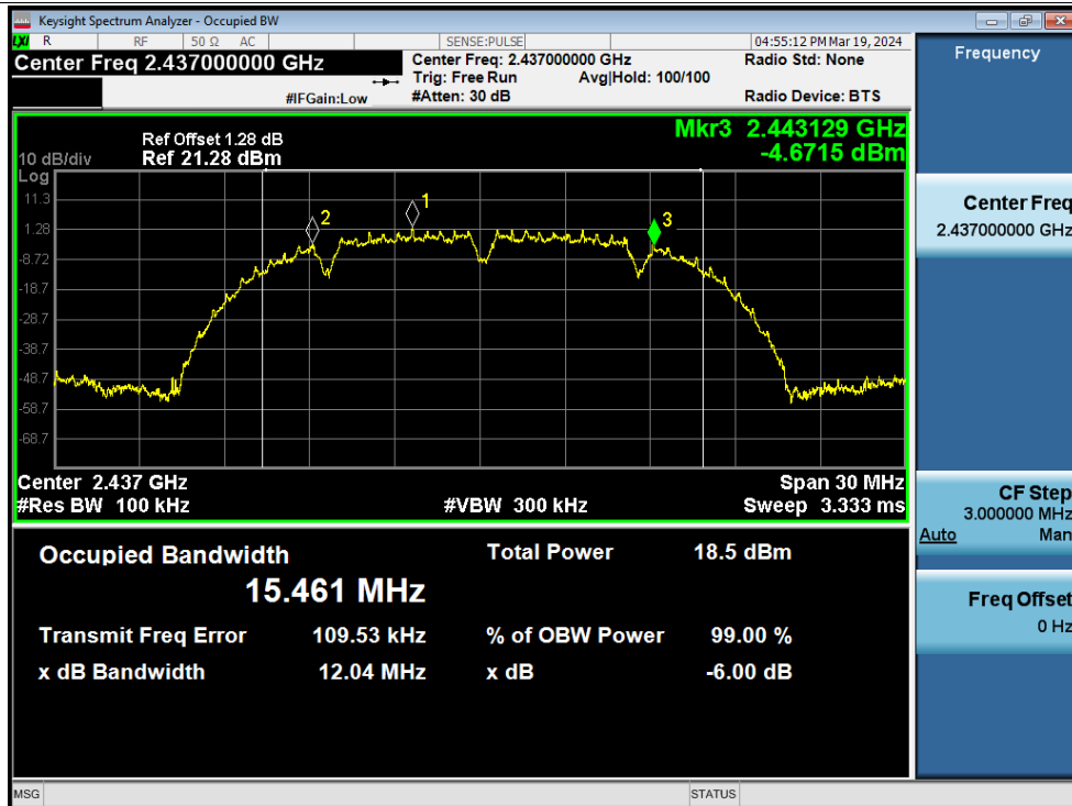
-6dB Bandwidth NVNT b 2437MHz Ant1
