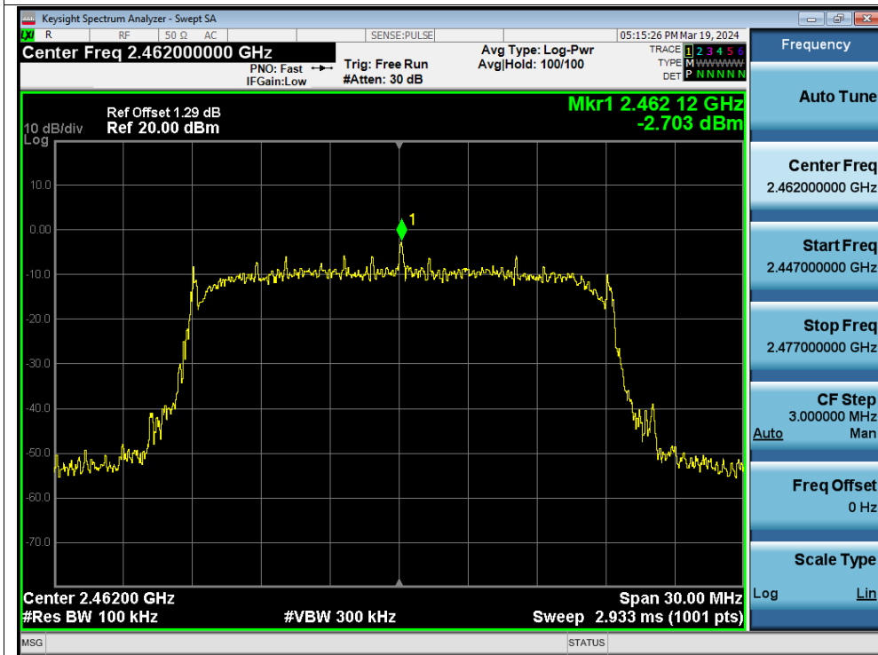
Tx. Spurious NVNT n20 2462MHz Ant1 Emission
