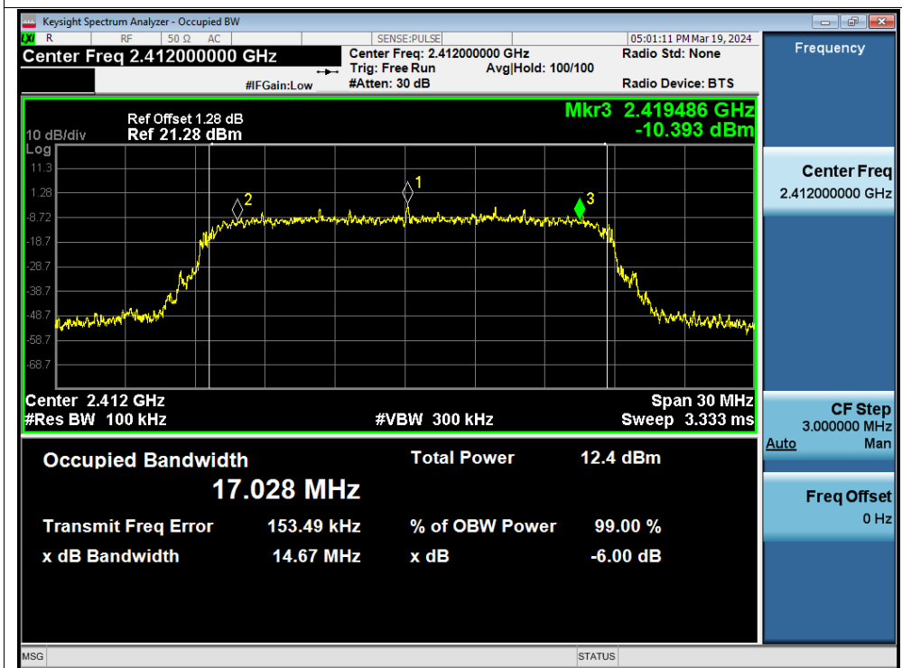
-6dB Bandwidth NVNT g 2412MHz Ant1
