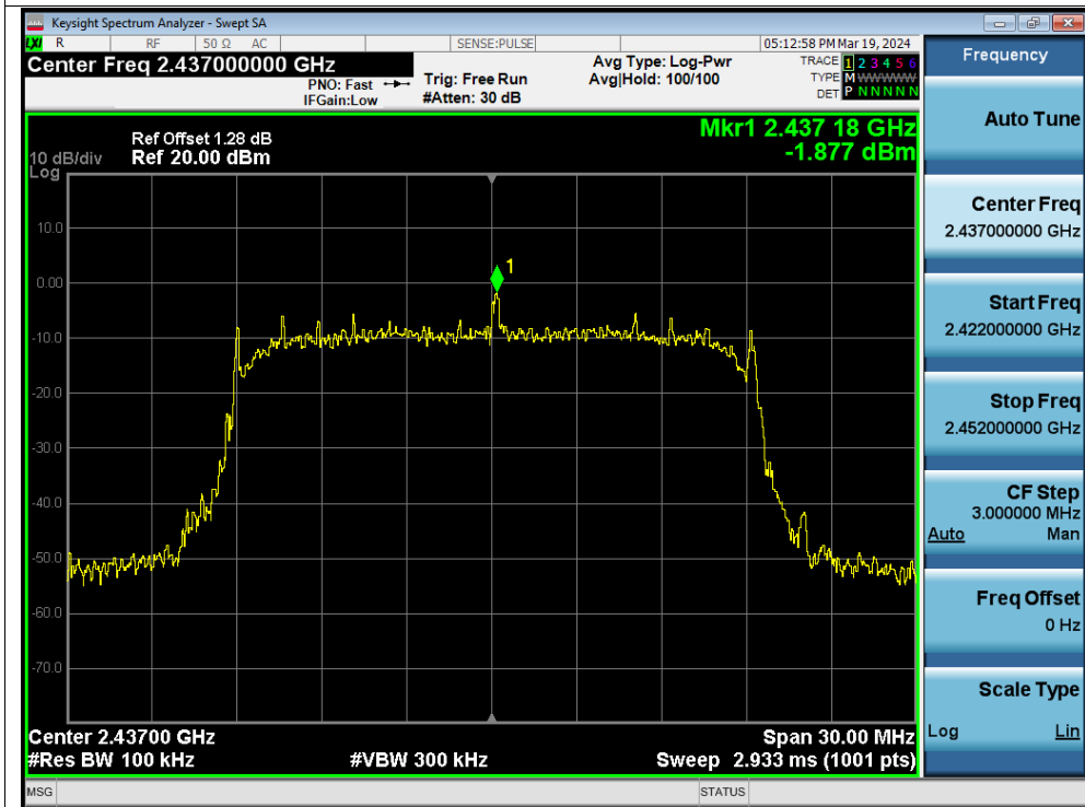
Tx. Spurious NVNT n20 2437MHz Ant1 Emission
