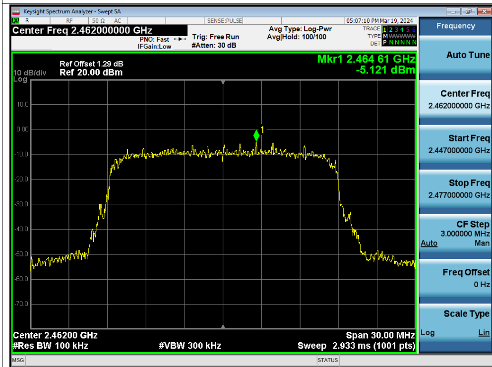
Tx. Spurious NVNT g 2462MHz Ant1 Emission
