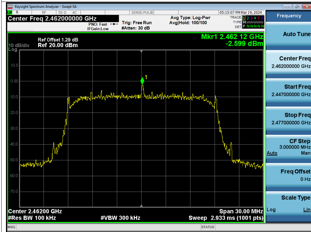
Band Edge NVNT n20 2462MHz Ant1 Emission
