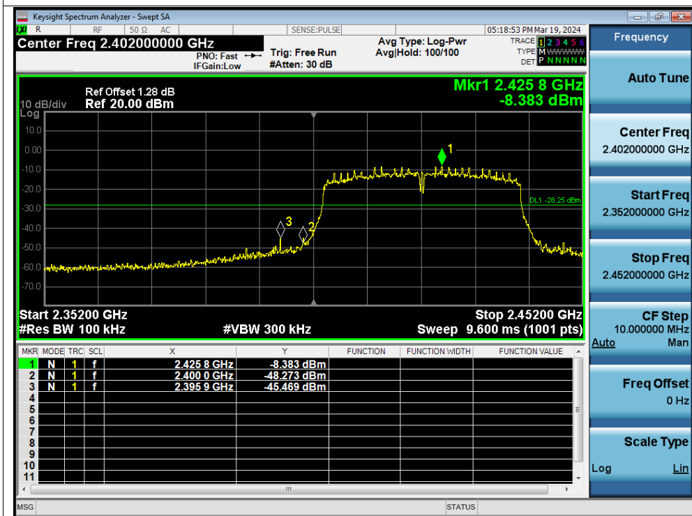
Band Edge NVNT n40 2422MHz Ant1 Emission
