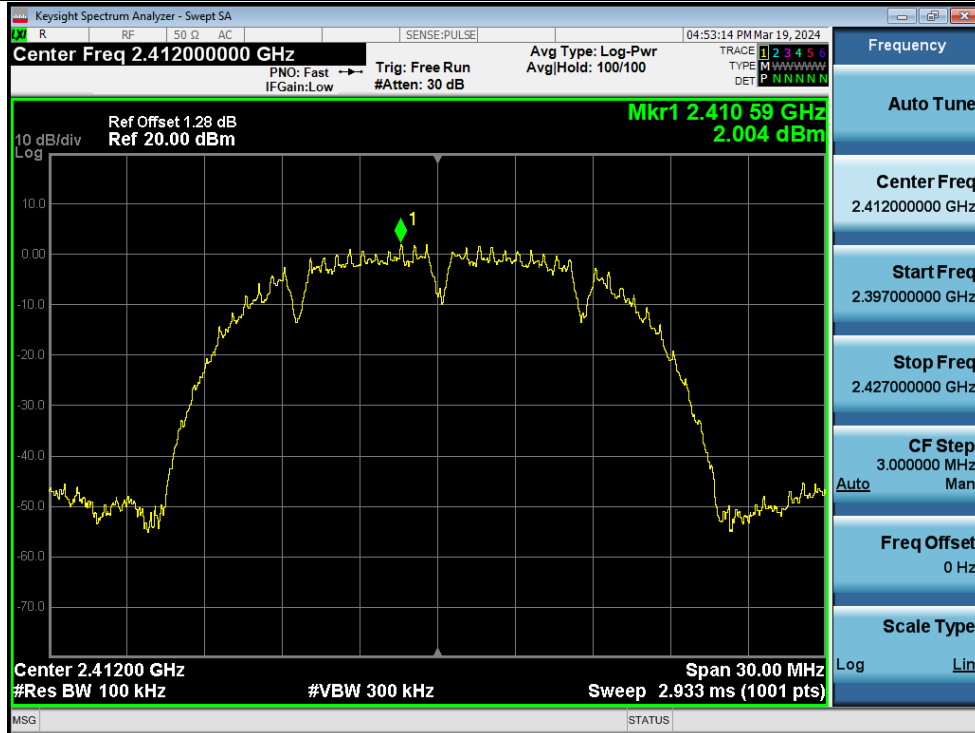
Tx. Spurious NVNT b 2412MHz Ant1 Emission
