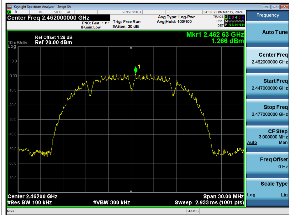
Tx. Spurious NVNT b 2462MHz Ant1 Emission
