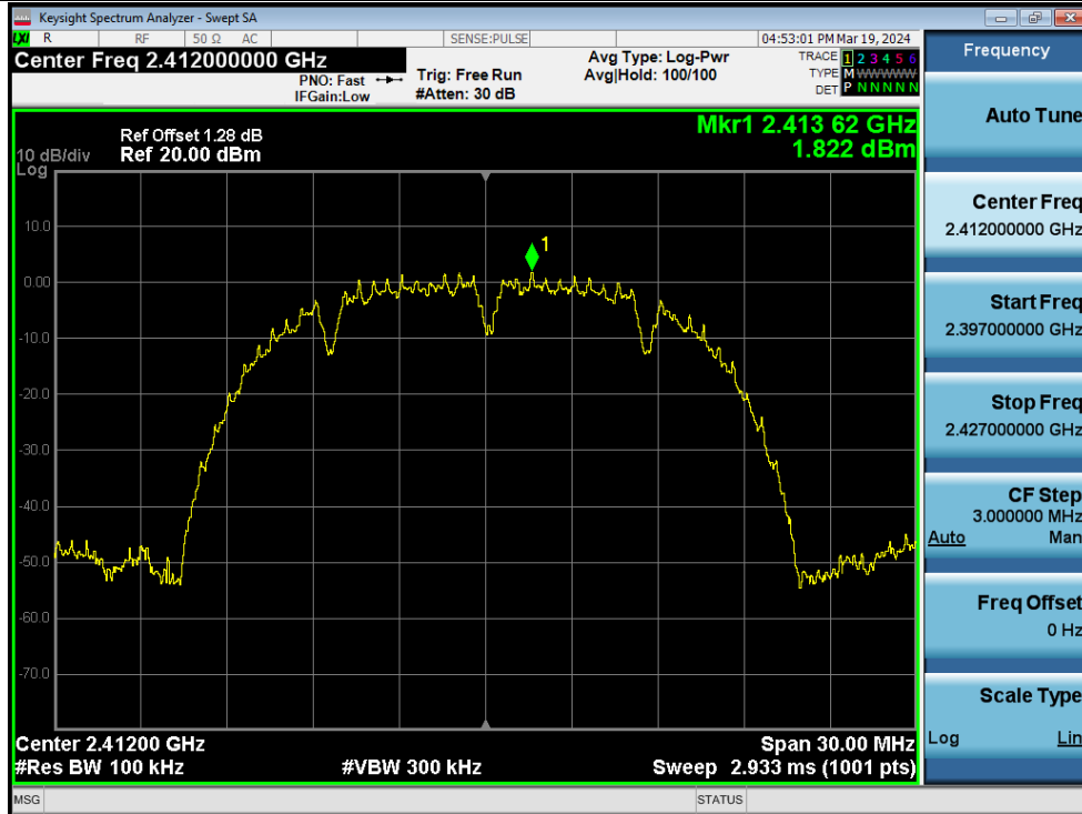
Band Edge NVNT b 2412MHz Ant1 Emission
