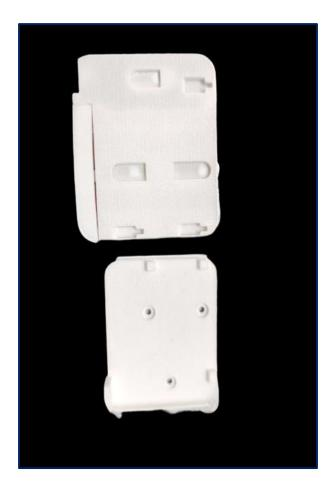
Measure the Device Position on the Cooler and mark to install the backplate into the Cooler. Slide up the SmartTagAON after removing the screw and, take out the device from the backplate.
