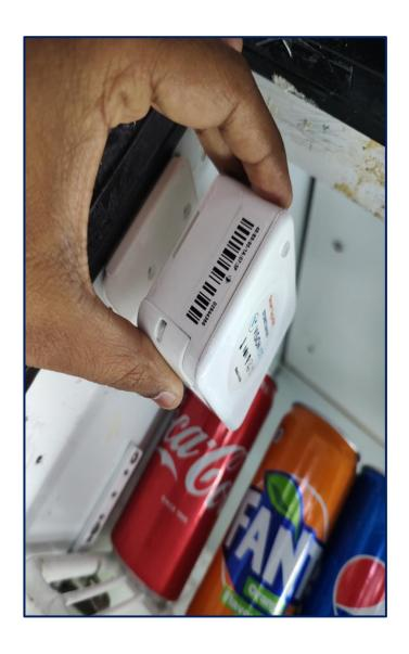
➤ Slide down the SmartTagAON Device in the backplate and tighten the backplate screw using the screwdriver.
