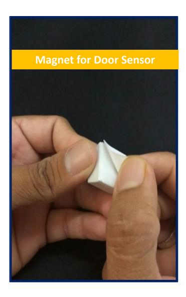
The magnet should be installed edge of the device and in front of the magnet sensor symbol.
